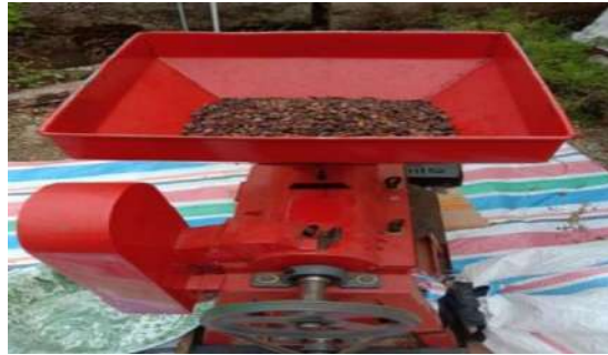
Figure 1. Sorting, separating the remaining coffee beans or dirt from coffee fruit skin waste using a sorting machine
