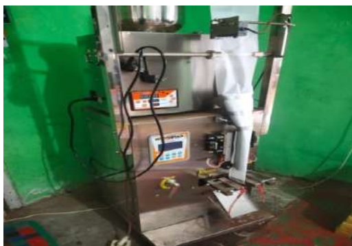
Figure 4.1. the process of filling tea powder into tea bags using a machine
